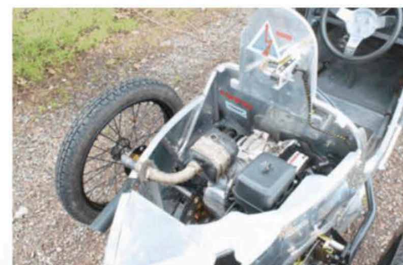
The mid-engined layout aids stability
